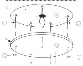
Remove rods ① and attach 🖯 to 🛆 with the button head screws ( )
